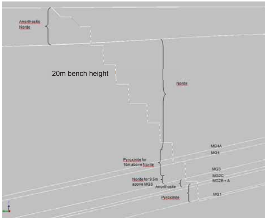
Figure 8.2.2_6 Diagram of the Proposed Highwall configuration showing Geology
