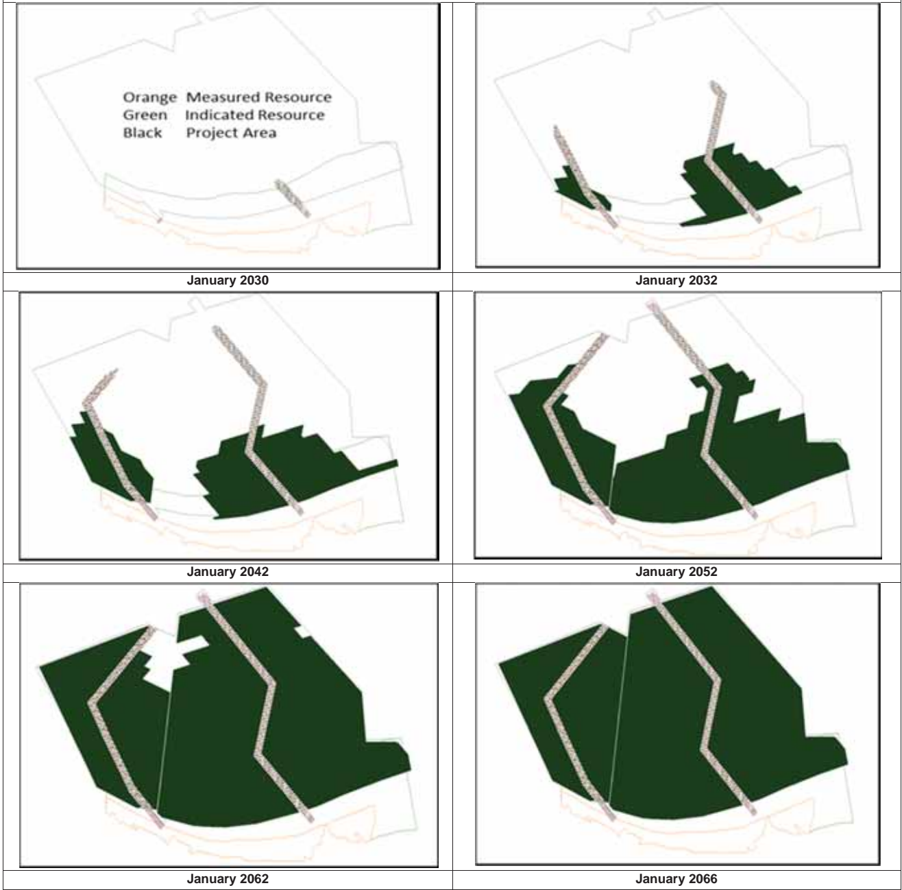
Figure 8.4.9_2 Underground Period Progress Plots: MG2 Chromitite Layer
